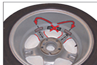
HID function for hidden weight mode behind spokes
