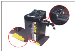
Break pedal and warning light
